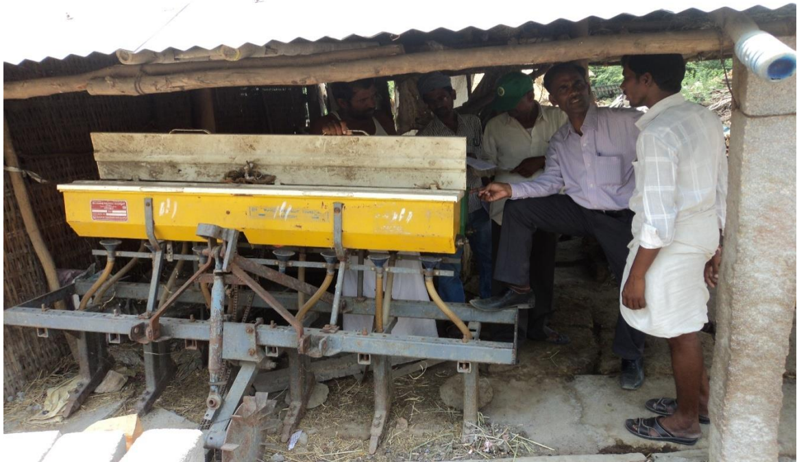
Survey team discussion with farmer about the maintenance of Seedcum fertilizer drill
